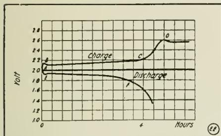
Fig. 3.—Curves Showing Change in Lead Storage Cell Potential on Charge and Discharge.
