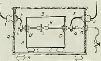
music strings are supported in the usual manner as indicated. At a point along each string is placed an electro-magnet which starts the string vibrating when its circuit is closed by the key contact shown. Included in this circuit is a special tuned interrupter or pulsator near the top of the string.
