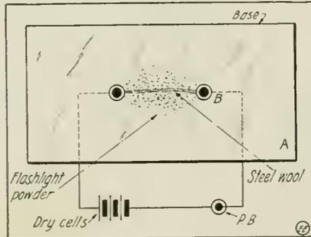
When Current From the Battery Is Past Thru the Single Strand of Steel Wool, It Becomes Incandescent; Igniting the Flashlight Powder.
