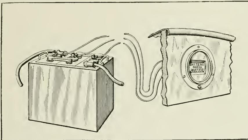
Every Battery User, and That Includes Most Every Autoist, Knows What a Nuisance It is to Keep Tabs on the Electrolyte Level. Here's An Instrument That Indicates Instantly When "Battery Needs Water."
