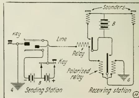
Connections for Original Edison "Quadruplex" Telegraph System.
