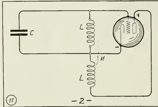
This Audion Diagram Represents Another Method of Coupling Inductively the Plate and Wing Circuit. In This Case Condenser C, Is Shunted Across the Wing Inductance Permitting Greater Freedom of Tuning Grid Current.
