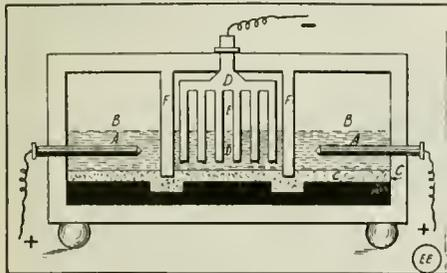
Fig. 88. Diagrammatic View of the Castner-Kellner Process for the Electrolytic Production of Caustic Soda and Caustic Potash.
