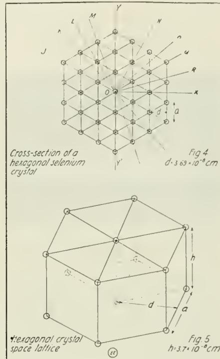
X-Ray Analysis Has Shown That the Selenium Atoms Are Situated at the Corners of Triangles, in Such a Manner as to Form Hexagons. The Distance Between Atomic Centers Is of Course Extremely Small.
