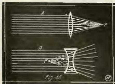
How Light Passes Thru a Convex Lens (A) and a Concave Lens (B). The Point "F" Is Called the Focal Point.
