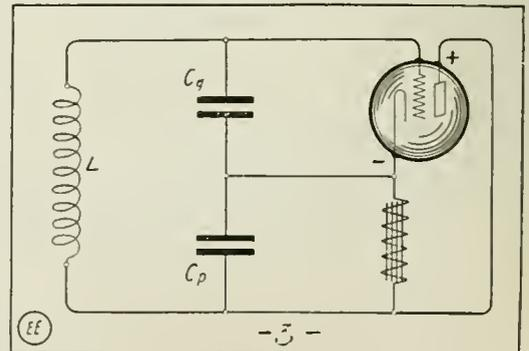
Diagram 3 Shows a Method by Which Plate and Wing Units Are Coupled Electrostatically Thru Condensers C<sub>g</sub> and C<sub>p</sub>.
