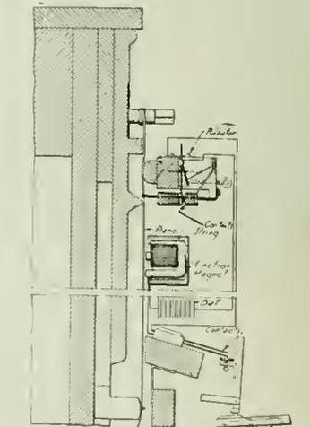
This is one of the cleverest electrical piano ideas we have seen. The music strings are supported in the usual manner as indicated. At a point along each string is placed an electro-magnet which starts the string vibrating when its circuit is closed by the key contact shown. Included in this circuit is a special tuned interrupter or pulsator near the top of the string.
