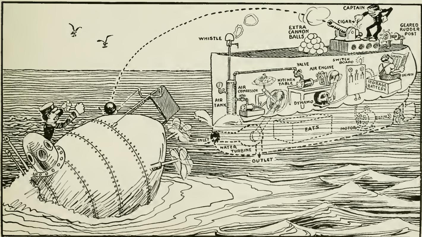
SELF-PROPELLED BOAT. Water Enters Ship's Bow Thru Inlet, Leaving It by Outlet, Incidentally Driving Water Turbine. The Latter Drives Air Compressor, Which Runs Air Engine and This Drives the Dynamo. The Latter Charges Storage Battery Which Runs Motor. Motor Operates Ship's Propeller, Thus Ship Will Never Run Out of Power. Inventor, Thomas Stewart, Jersey City, N. J.
