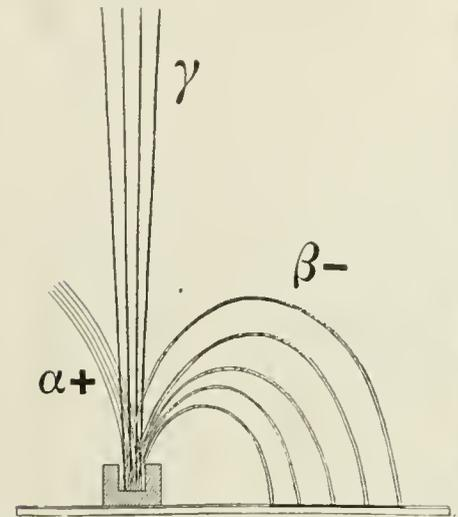
Showing the Separation of the Three Entirely Different Types of Radium Emanation Rays in a Strong Magnetic Field.
